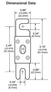
CATALOG SYMBOL: ANL NON-TIME DELAY 32 VOLTS AC 35 TO 750 AMPERES U.L. RECOGNIZED
