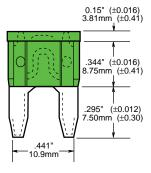
CATALOG SYMBOL: ATM FAST-ACTING 2 TO 30 AMPERES 32 VOLTS DC
