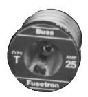
CATALOG SYMBOL: T DUAL-ELEMENT, TIME-DELAY 1 TO 30A 125VAC OR LESS U.L. LISTED
