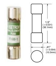
CATALOG SYMBOL: FNM TIME-DELAY 1/10 TO 30 AMPERES INTERRUPTING RATING - SEE CHART BELOW UL LISTED: STD. 248-14, 0-10/250V AC; 12-15/125V AC FILE #E19180, GUIDE #JDYX CSA CERTIFIED: 1-10/250V AC; CLASS 1422-01, 12-15/125V AC; FILE 53787 DC RATING: 1-15A rated 125V DC and 1.6 KAIC.
